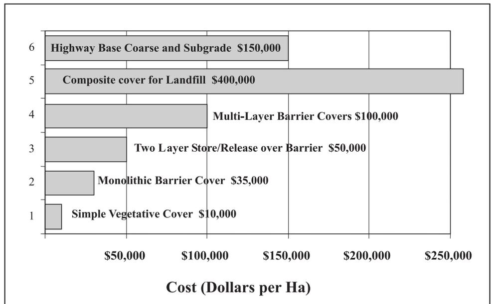
Figure 8: Indicative costs for cover construction. Dollar amounts are approximate for construction in Australia, Canada and the United States, in local currency.
