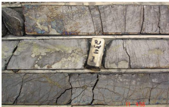
Figure 6. Detailed photograph of sampled massive sulphide core indicating the extent of micro-fracturing/defects.
